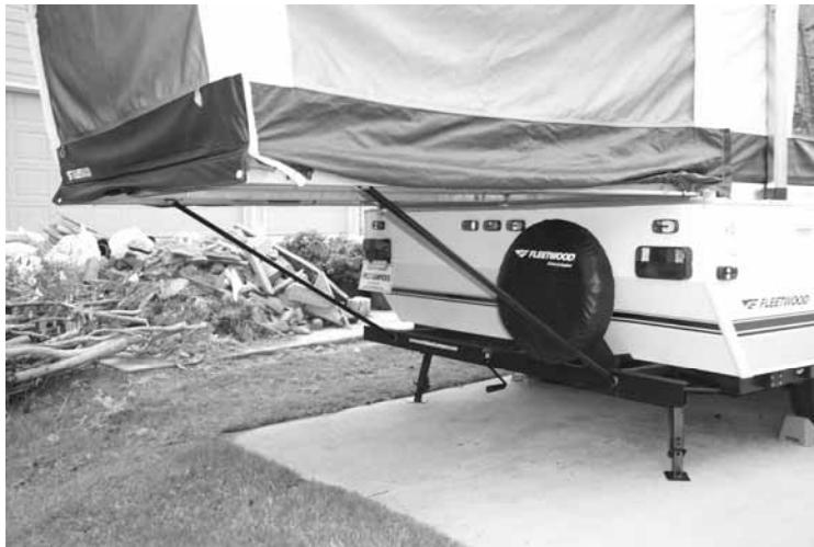
Raise and stow bed support rails. Slowly push in rear bed. Fold tenting neatly on top of bed as it slides in.
