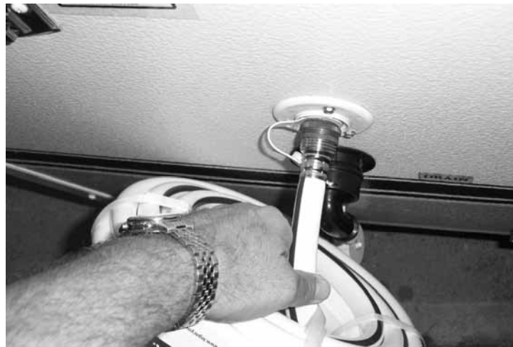
Hook up water hose and regulator here.
