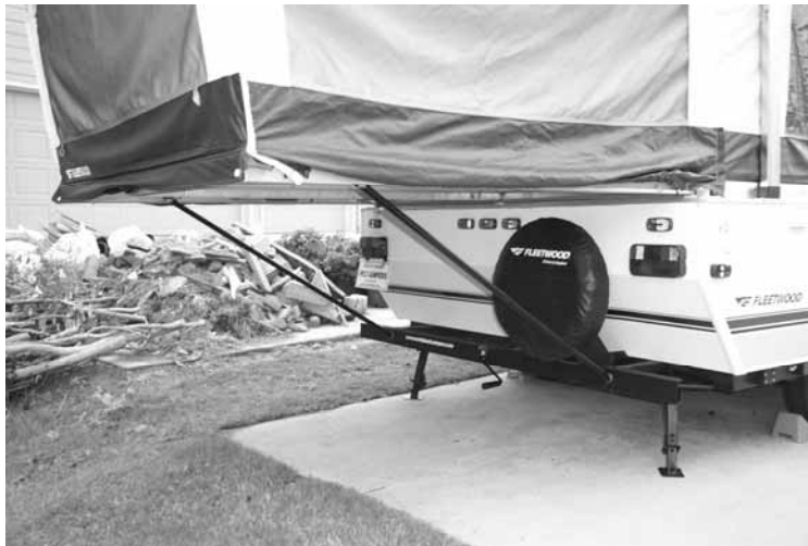
Pull out rear bed and lower bed support rails. Attach to bumper studs.
