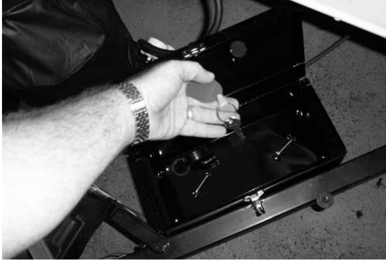
Get Key, Wheel Chocks, Lug wrench, and jack handle from Tongue Tool Box.
