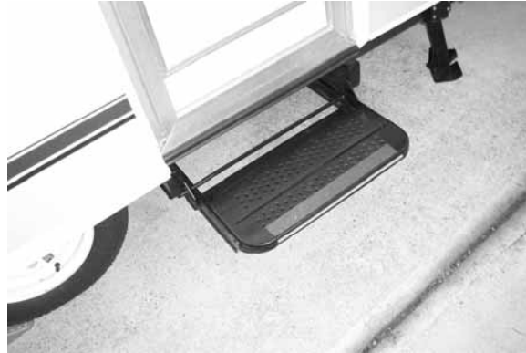
Door step in lowered position.
