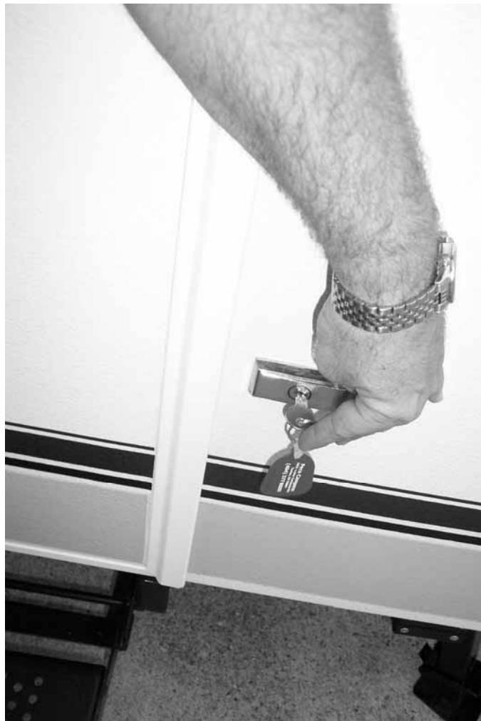
Before lowering roof, close lower door.
