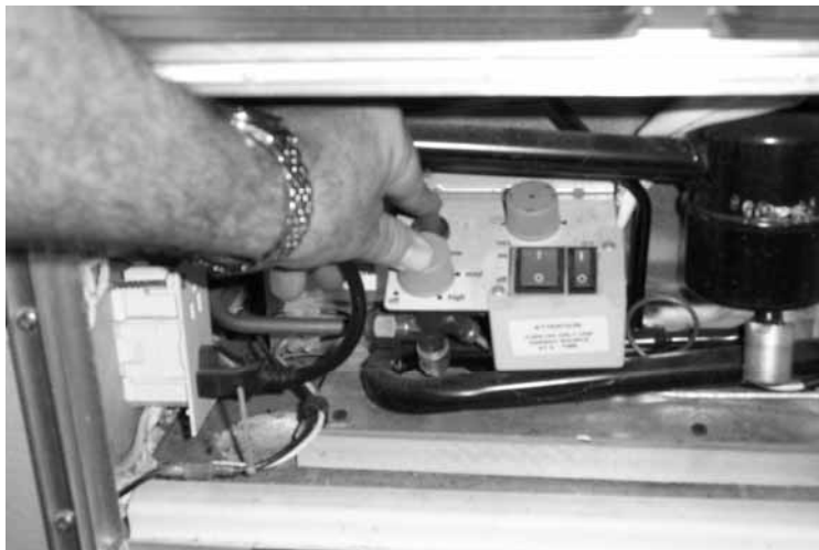
To run Refrigerator on Propane, Turn on Gas knob, Press and hold Grey knob and press Red igniter repeatedly until it lights.
