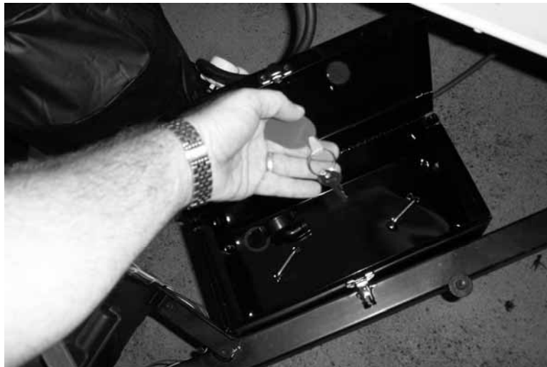
Place Key, Wheel Chocks, Lug wrench, and jack handle in Tongue Tool Box.
