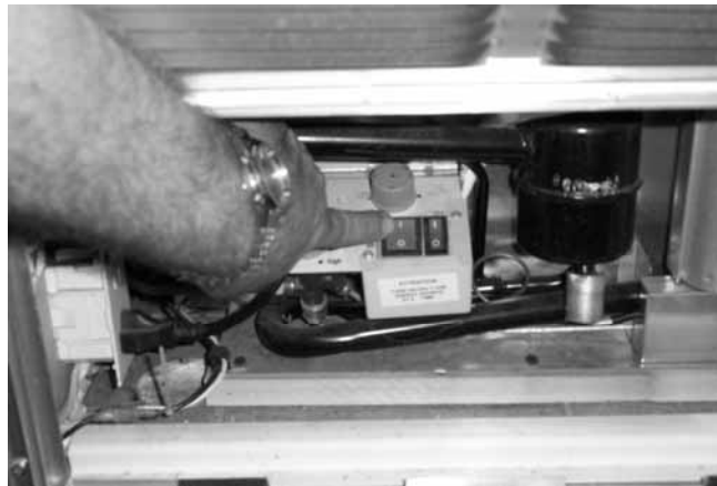
To run Refrigerator on 120V Electric, press green switch to "ON"
