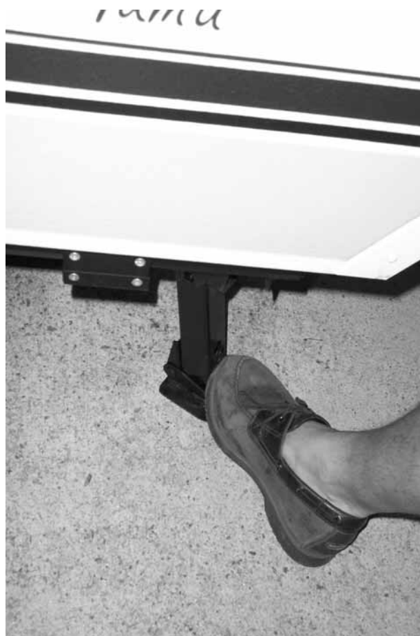
Before lowering roof, release all jacks.
